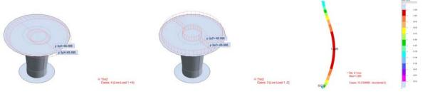
Loads applied to the bottom of mouse hole
