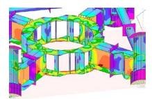
Stress Plot of Wellhead Spider Frame
