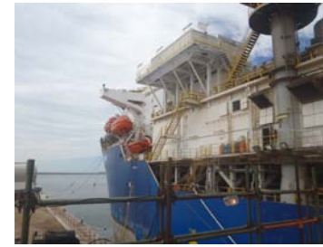
Temporary living quarter
